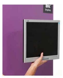
**3** Mount the screen (see photo instruction B) and then push the screen holder into the post holder while at the same time pressing the two buttons on the post holder together.
