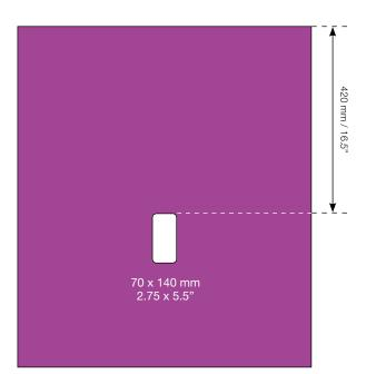
Make a 70 x 140 mm / 2.75 x 5.5" hole in the center of and 420 mm / 16.6" from the top.
