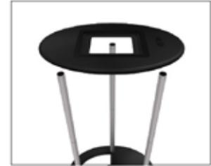
4. Place counter top onto poles. Tap down with hand to secure.
