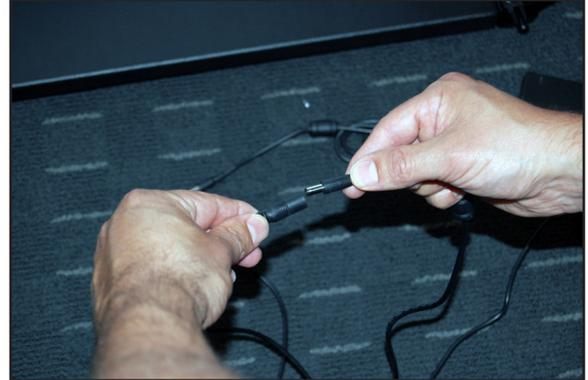
4. At the back of the display connect the two cords from the bottom of the lightbox into the power supply cords. Then plug into your electric source and turn on.
