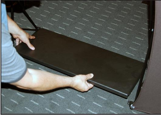
1. Set up all 1x3 Xpressions® SNAP!™ frames and connect them together with a CONNEX™ shelf top and bottom.
